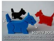
In this case Scotty Dogz will easily fit on the build plate. He will print in about 52 minutes and use 7.63 grams of filament to create. Filament is 10 cents per gram so Scotty Dogz will cost 70 cents to print.
